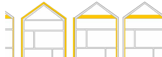
Ensuring continuous insulation
